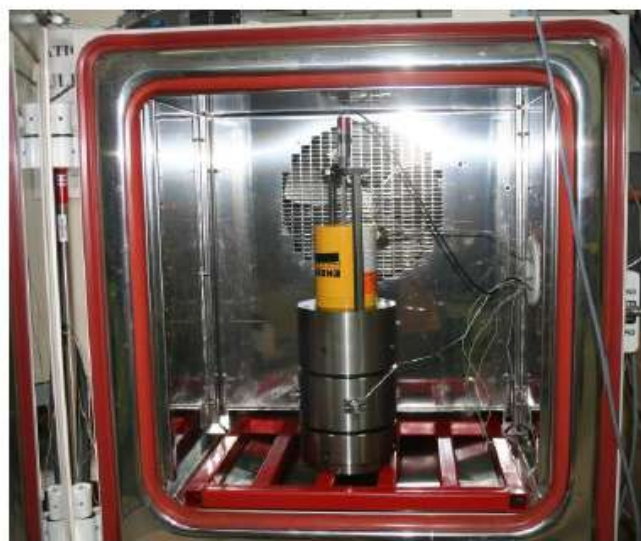
Artificial ground freezing (thermo-mechanical) test
